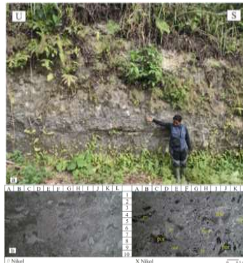
Figure 10. observation location LP 15 a. human scale outcropping, b. Packstone is composed of large (for) which has been partially replaced by pseudosparite with carbonate sludge (cmd) which is replaced by microsparite (msp), present dissolved cavity (por).
